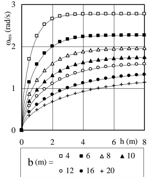
Figure 3: Lowest tank resonance frequency as a function of water depth  $h$  for several tank width values  $b$ .
