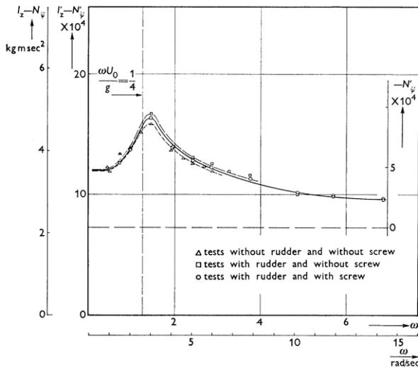
Figure 4: Influence of  $\omega_3'$  on added moment of inertia from PMM yaw tests (van Leeuwen, 1964)
