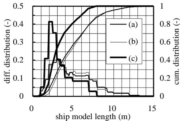
Figure 1: Differential and cumulative distribution of the length of ship models used for several types of captive model tests (22<sup>nd</sup> ITTC Manoeuvring Committee, 1999)
